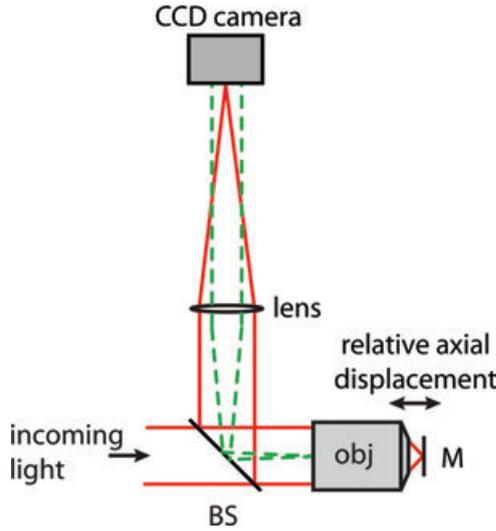
**Fig. 1.** Typical setup for PSF measurement and subsequent electric field retrieval. BS, plate beamsplitter. Red, light path. Dotted green, pupil and conjugated planes.
