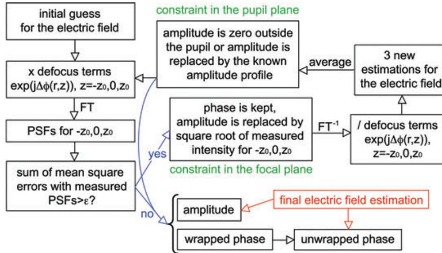
Fig. 2. Flow diagram of the electric field retrieval algorithm. See section 3 for typical values of the different parameters.
