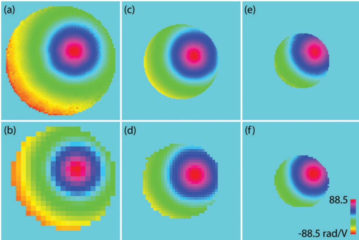
**Fig. 6.** Influence function of an actuator of the pupil-plane-conjugated DM on the phase in the pupil plane of various objectives, as measured using phase retrieval (top) and a SHS (bottom). First column, 20 $\times$ , 0.75NA air objective; second column, 10 $\times$ , 0.25NA air objective; third column, 60 $\times$ , 1.2NA water-immersion objective. All profiles are displayed using the same colour scale.
