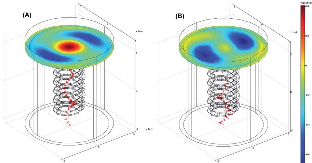
Fig. 5. (Color online) FEM simulations of the optical activity in a metallic helix in the terahertz domain. Color map provides the value of the electric field along the  $x$  axis, for right (A) and left (B) incident circular polarizations. The color scale is identical for both polarizations. The red arrows show the electric field direction at the center axis of the helix.
