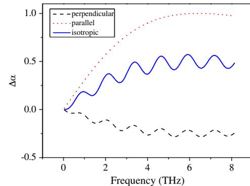
Fig. 4. (Color online) Circular dichroism in arbitrary units as a function of the frequency for helices whose axis is perpendicular (dotted line) and parallel (dashed line) to the beam propagation and for an isotropic distribution of helices (solid line). Note that the isotropic signal goes to 0 when the frequency becomes very small, corresponding to the validity regime of the usual multipolar expansion.
