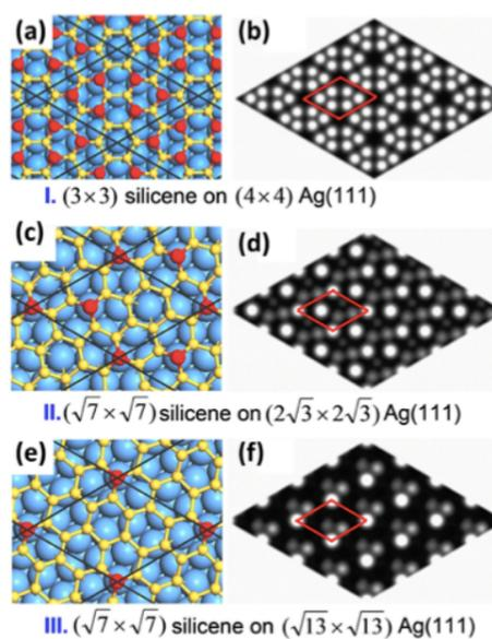
Fig.3 (a),(c),(e) Atomic structures of three types of silicene on Ag(111) superstructures and (b),(d),(f) their corresponding STM images [7].
