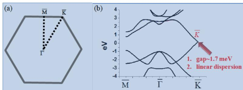
Fig.2 (a) Schematic of the first Brillouin Zone of silicene and its points of high symmetry. (b) Band structure of silicene. Zero of energy set at the Fermi level. There is a small band gap at K and bands are linear near the cross section point K.
