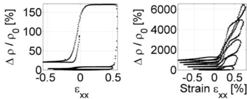
**Figure 4:** Relative change of resistivity as a function of the strain component  $\epsilon_{xx}$  for indium tin oxide (left) and aluminum doped zinc oxide (right)
