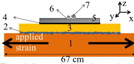
**Figure 1:** Cross section of the layer stack: 1: 5 mm thick PVD substrate, 2: alkyl cyanoacrylate adhesive, 3: 50  $\mu\text{m}$  polyimide foil, 4: 150 nm SiNx, 5: semiconducting layer, 6: evaporated aluminum contacts, 7: conductive epoxy adhesive to attach wires.
