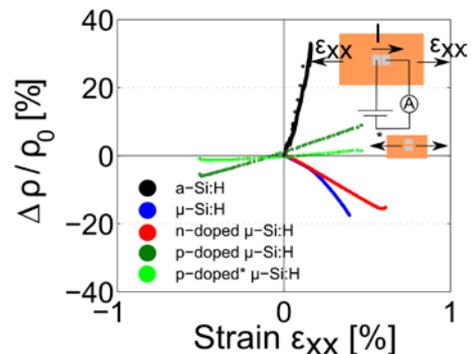
**Figure 3:** Relative change of resistivity as a function of the strain component  $\epsilon_{xx}$  for silicon based materials
