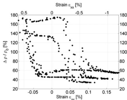
**Figure 6:** Relative change of resistivity as a function of the strain component  $\epsilon_{xx}$  and  $\epsilon_{yy}$  in the A2 configuration for ZnO:Al. The applied strain and the current are perpendicular to each other. The decisive strain component is thus the one parallel to the current flow:  $\epsilon_{yy}$
