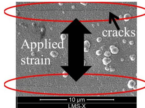
**Figure 8:** In-situ SEM image during the mechanical stressing of a n-doped  $\mu$ -Si:H. The resistivity is measured simultaneously. Cracks are visible after applying a tensile strain of X%.
