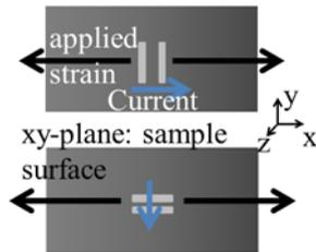
**Figure 2:** Schematic top view of the sample. The rectangular contacts (10 mm x 5 mm, 1 mm distance) are placed in such a way that the current is flowing either parallel (upper drawing, called A1 configuration) or perpendicular (lower drawing, called A2 configuration) to the applied strain.
