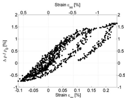
**Figure 5:** Relative change of resistivity as a function of the strain component  $\epsilon_{xx}$  and  $\epsilon_{yy}$  in the A2 configuration for ITO. The applied strain and the current are perpendicular to each other. The decisive strain component is thus the one parallel to the current flow:  $\epsilon_{yy}$
