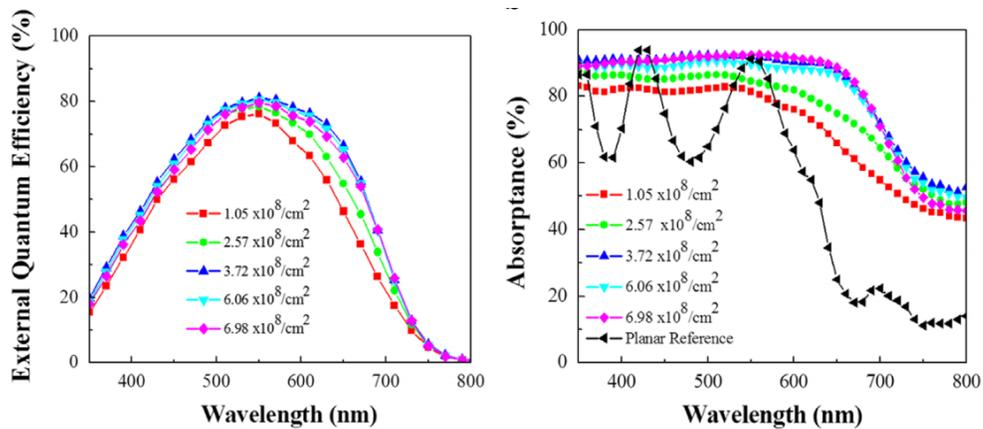
**Figure 1.** Left: Measured external quantum efficiency of different radial junction solar cells as a function of the wavelength. Right: Measured total absorbance of the same solar cells as a function of the wavelength.
