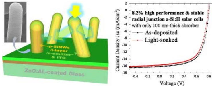
**Figure 1.** *Left:* Schematics of radial junction solar cells. *Right:* Example of measured J-V characteristics and corresponding performance of a solar cell before and after the light soaking.
