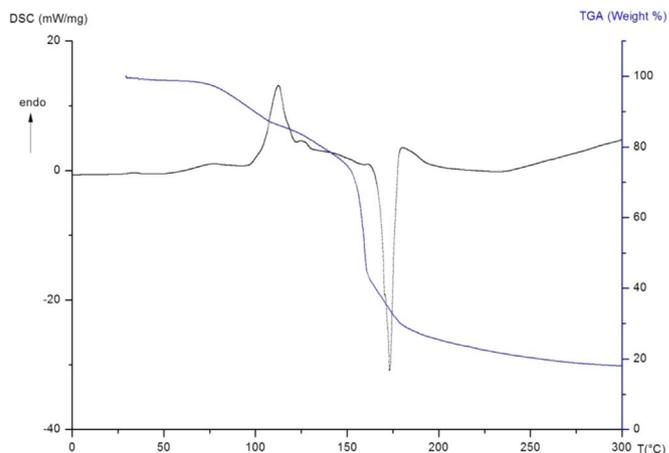
Fig. 4. TGA and DSC thermograms of the DOTN crystal.
