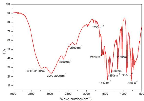
Fig. 2. FTIR spectrum of DOTN crystal.
