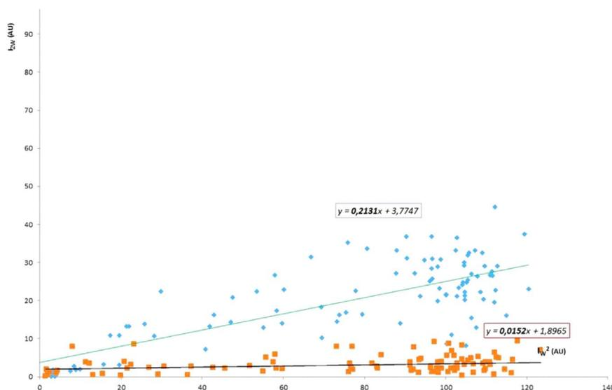
Fig. 9. Power dependence of  $I_{2\omega}$  vs.  $I_{\omega}$  for nitrate and water.
