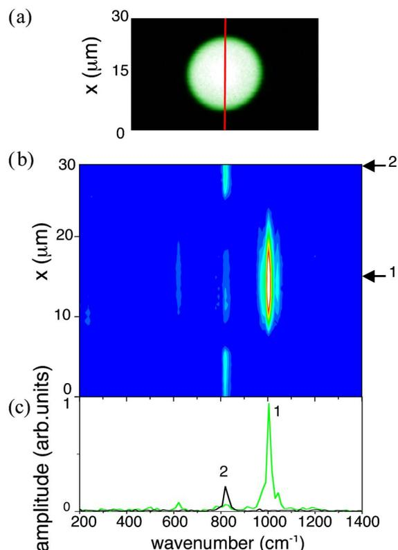
Fig. 2. (Color online) (a) Two-photon fluorescence image of a  $20\text{ }\mu\text{m}$  polystyrene bead immersed in 2-propanol. (b) Spectrally resolved FTCARS image of the line in (a) [see (c) for scale]. (c) CARS spectra at positions 1 and 2 in (b).
