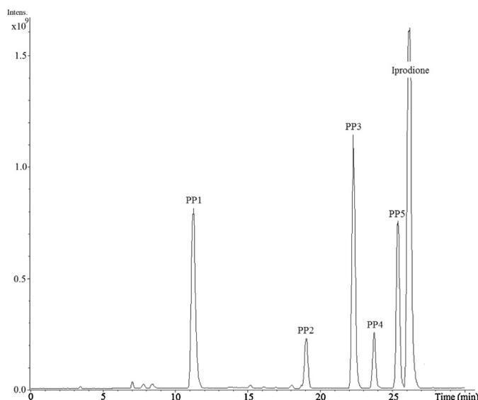
**Fig. 2.** LC–MS chromatogram of the aqueous solution of iprodione irradiated for 60 min (ESI in the positive mode, fullscan detection).
