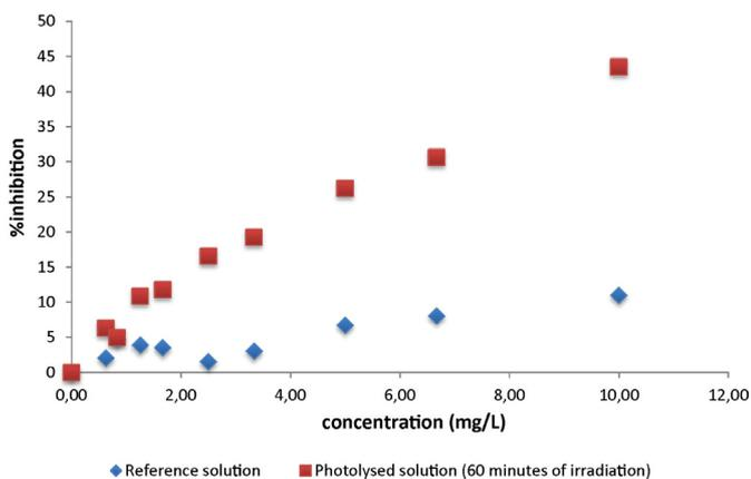
**Fig. 5.** Response–dose curves for both reference and photolyzed iprodione solutions with the *Vibrio fischeri* bioluminescence inhibition test.
