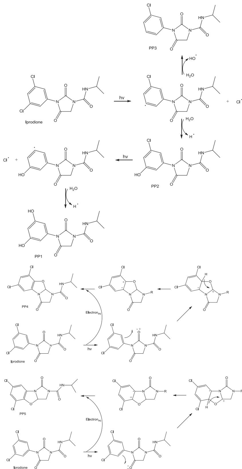
**Fig. 3.** Suggested transformation pathways of iprodione under UV-vis irradiation.
